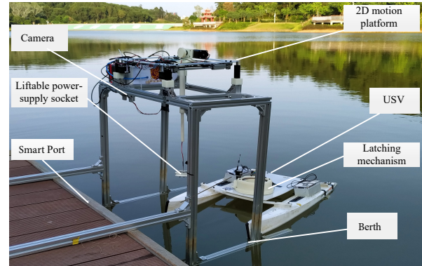
Fig. 1. A USV docks at the berth and performs the automatic latching and charging operation for further tasks in a berth.
